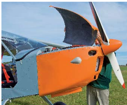
Simple glass fibre cowlings are easily removed for daily inspection
