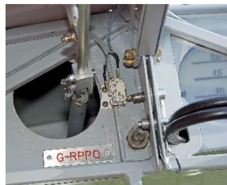
Microswitches trigger an audible alarm if spar pins are not fully home
