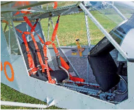
Front seat hinges forward for easy access to rear through very large door
